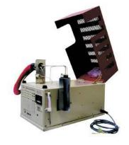
gas out. A single contact closure from the host's data system or GC initiates the mechanical agitation of the heated VOA vial sleeve, as required by Method 5035.
